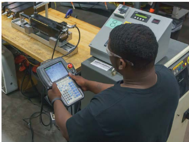
Final system test ensures the feedback device is properly aligned with the ServoWeld motor poles.
